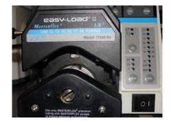
Figure 1: EZ Load II Peristaltic Pump Head
