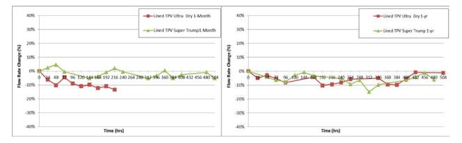
Figure 8: Effect of chemical exposure and time on lined thermoplastic vulcanizate (lined TPV) tubing performance
