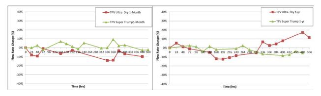
Figure 7: Effect of chemical exposure and time on thermoplastic vulcanizate (TPV) tubing performance
