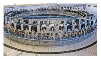
Rotary milking parlors were designed to automate the milking process and to decrease milk's contact with humans and air, which can cause premature spoiling. Milking parlor tubing plays a major role in safely transporting the milk from the cow to the consumer. Milking a large number of cows successively and automatically can boost productivity but it should not impact safety.
